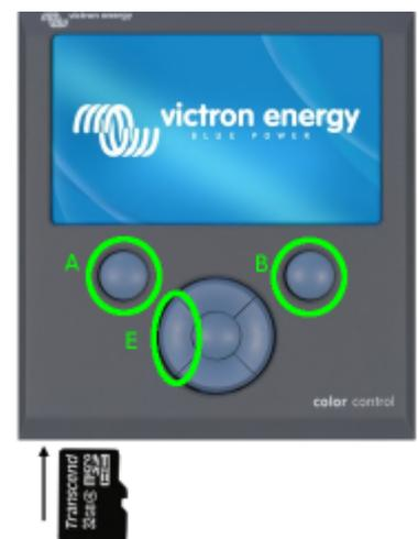
1. Get a microSD card. The card needs to be formatted with either a FAT or FAT32 file system. Preferably use a card of 32GB or smaller, as larger cards are often hard to format with mentioned FAT filesystems. The upgrade requires less than 150MB on the card.
