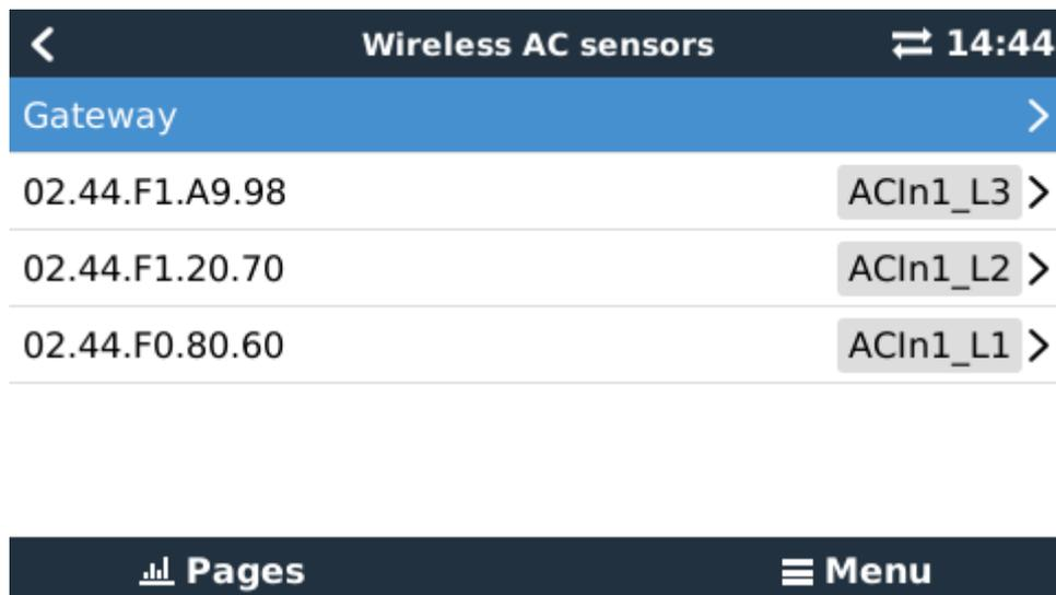
Select a sensor to assign a location to it. For example AC-In1\_L3.
