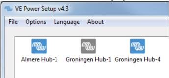
5. After selecting the site, VE Power Setup will establish communication to the selected site. Once established, it will perform a remote scan, to find all products connected to the Color Control. Now select the product you want to configure:
