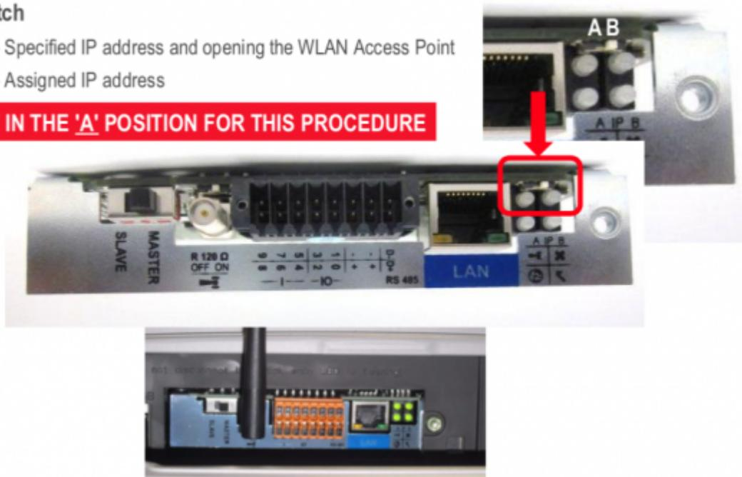
2. Connect both, the Fronius and the CCGX, on the same LAN network, either directly with a LAN cable or using a network switch.
