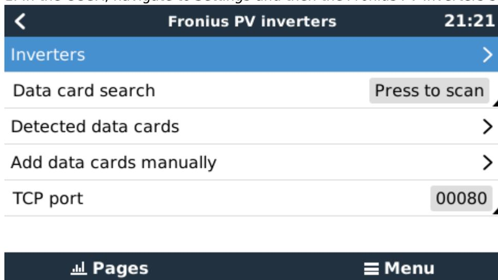
2. Select *Scan* in the CCGX menu, and after completion go into the *Inverters* submenu to see the results. If scanning does not find the inverter, manually add the IP address of the Fronius Datamanager from its card, or box.
