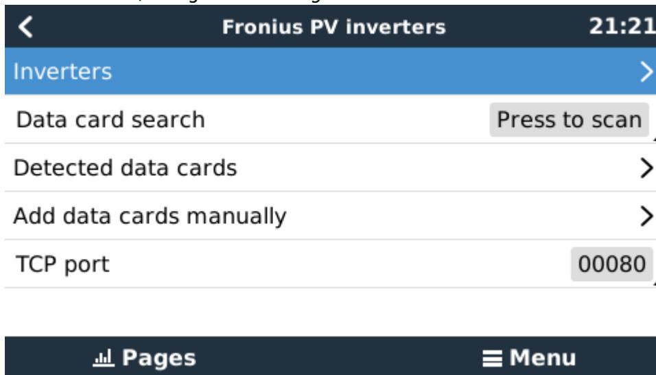
2. Select *Scan* in the CCGX menu, and after completion go into the Inverters submenu to see the results. If scanning does not find the inverter, manually add the IP address of the Fronius Datamanager from its card, or box.
