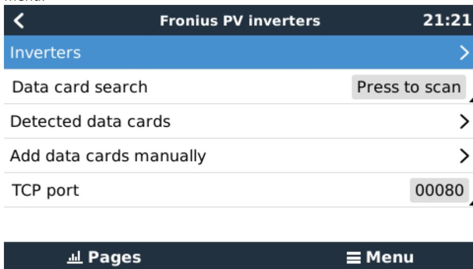
4. Select *Scan* in the CCGX menu, and after completion go into the *Inverters* submenu to see the results. If scanning does not find the inverter, manually add the IP address of the Fronius Datamanager from its card, or box.
