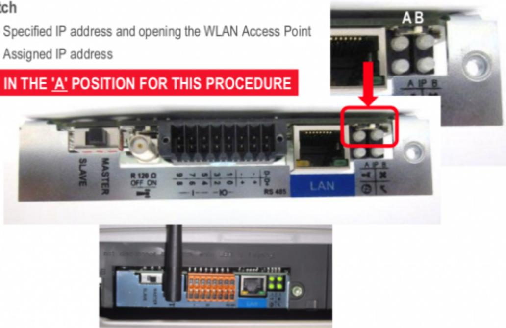
2. Connect both, the Fronius and the CCGX, on the same LAN network
