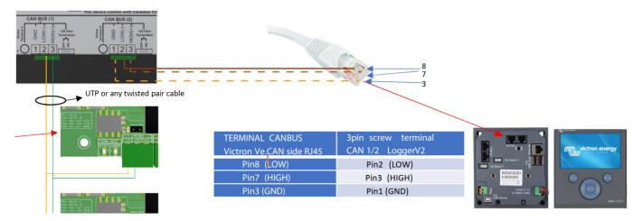
Then, plug a VE.Can terminator in the other VE.Can socket on the GX device alternatively, you can use the termination on the Logger V2 side. Two VE.Can terminators are included with the package of the GX device as an accessory, only one is used. Keep the other one as a spare.
