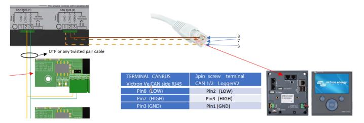
Then, plug a VE.Can terminator in the other VE.Can socket on the GX device alternatively, you can use the termination on the Logger V2 side. Two VE.Can terminators are included with the package of the GX device as an accessory, only one is used. Keep the other one as a spare.
