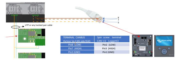
Then, plug a VE.Can terminator in the other VE.Can socket on the Venus-device alternatively, you can use the termination on the Logger V2 side. Two VE.Can terminators are included with the package of the Venus-device as an accessory, only one is used. Keep the other one as a spare.
