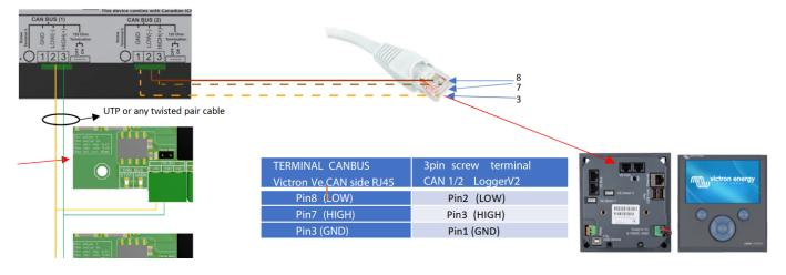
Then, plug aVE.Can terminator in the other VE.Can socket on the Venus-device alternatively, you can use the termination on the Logger V2 side. Two VE.Can terminators are included with the package of
