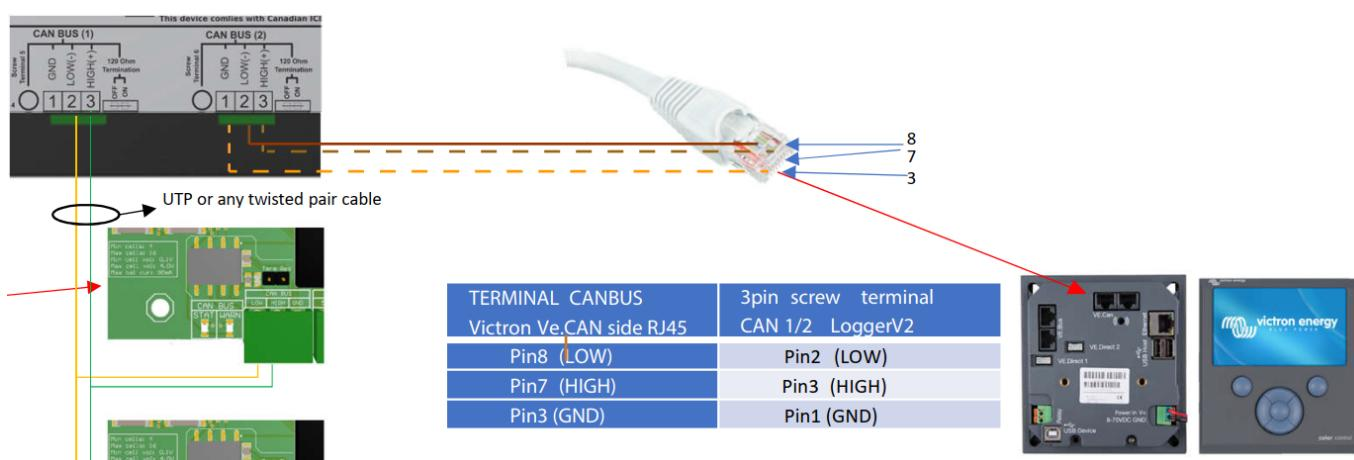
Then, plug a [VE.Can terminator](#) in the other VE.Can socket on the [Venus-device](#) alternatively, you can use the termination on the Logger V2 side. Two VE.Can terminators are included with the package of
