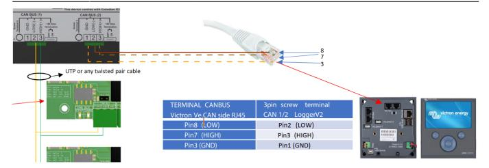
Then, plug aVE.Can terminator in the other VE.Can socket on the Venus-device alternatively, you can use the termination on the Logger V2 side. Two VE.Can terminators are included with the package of the Venus-device as an accessory, only one is used. Keep the other one as a spare.
