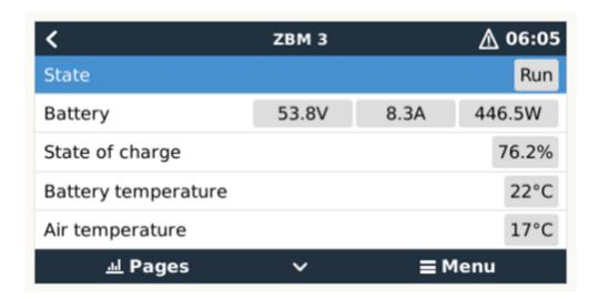
1. Connect the CCGX to each battery in the system via Modbus-RS485, (our RS485 to USB interface is needed for that, ASS0305700xx).
