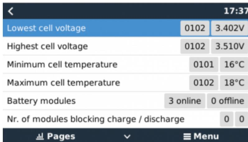
The prefix number to the cell voltages and temperature is used to identify which specific battery in the installation is reporting.
