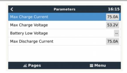
This parameters page is also a good place to check that all batteries are connected and working properly. In see the individual battery data sheet for the normal working conditions, e.g. the current limit per cell. For example, If each battery is rated to 25A charge current, and the menu shows a 75A charge current limit (75/25 = 3) means there are 3 Pylontech battery modules connected.
