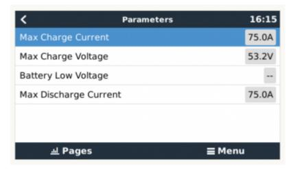
This parameters page is also a good place to check that all batteries are connected and working properly. In normal working conditions, the current limit is 25A per cell. For example, 75A charge current limit (75/25 = 3) means there are 3 Pylontech battery modules connected.
