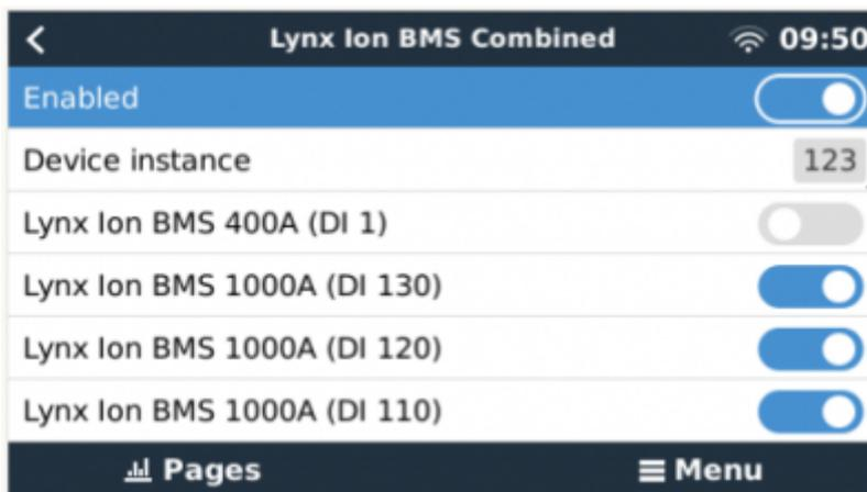
The new combined battery will be created in the device list and can be selected as the battery monitor to have parameter control by DVCC. If one of the Master LV's (Lynx BMS) fails, the system will stay active and keeps operating.
