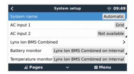
The combiner can be enabled in the System Setup menu. The Master LV's (Lynx Ion BMS) which need to be combined can be selected. The new combined battery can be given a new device instance. This will make it also available and can be easily identified on the VRM portal.
