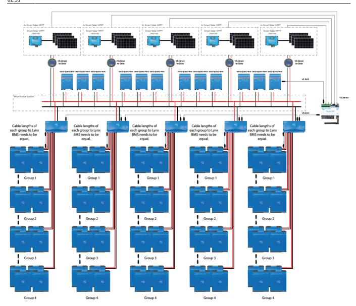
The GX products redundant/combined battery support
