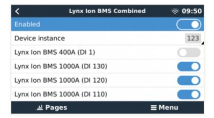
The new combined battery will be created in the device list and can be selected as the battery monitor to have parameter control by DVCC. If one the Master LV's (Lynx BMS) fails, the system will stay active and keeps operating.
