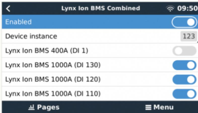
The new combined battery will be created in the device list and can be selected as the battery monitor to have parameter control by DVCC. If one the Master LV's (Lynx BMS) fails, the system will stay active and keeps operating.
