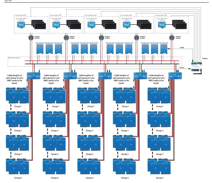
The GX products redundant/combined battery support
