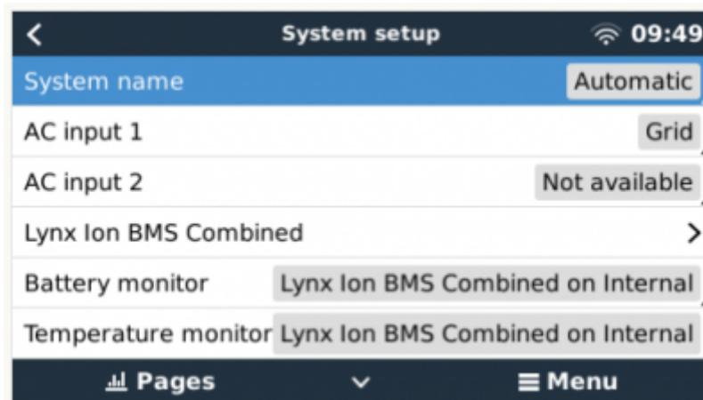
The combiner can be enabled in the System Setup menu. The Master LV's (Lynx Ion BMS) which need to be combined can be selected. The new combined battery can be given a new device instance. This will make it also available and can be easily identified on the VRM portal.
