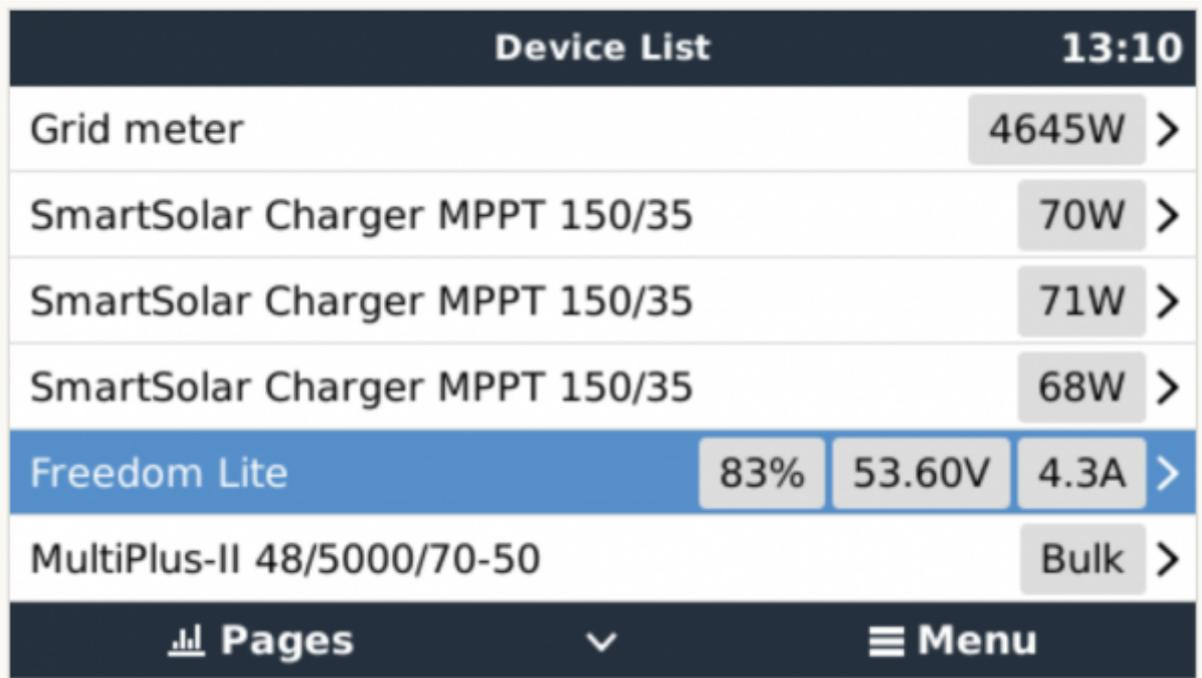
Freedom Lite → Parameters → Confirm that the Charge Current Limit and Discharge Current Limit are as per the Lite specifications.
