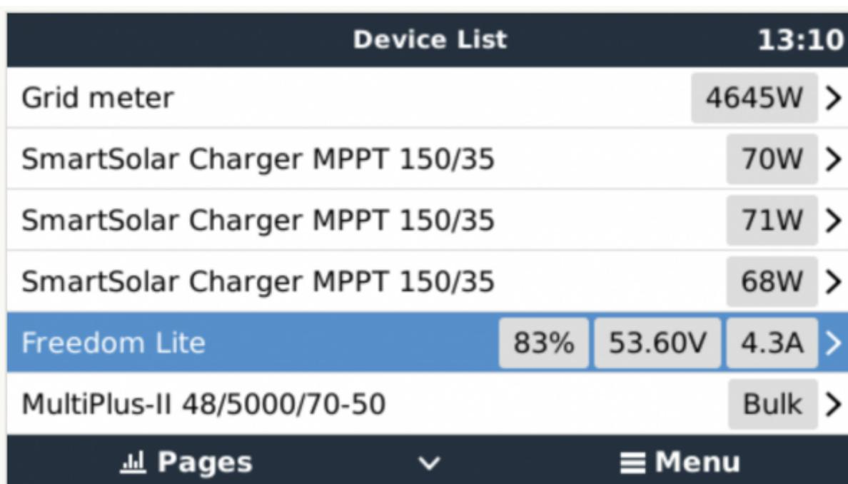
Freedom Lite → Parameters → Confirm that the Charge Current Limit and Discharge Current Limit are as per the Lite specifications (Note: if the battery is fully charged the CCL may be reduced. Check that the voltage target is within the range 54.8V to 55.8V (Note: below about 95% SoC the value reflected should be 55.7 or 55.8V. For a fully charged battery this value should range from 55.0V to 55.8V depending on the state of balancing of the cells in the Lite.
