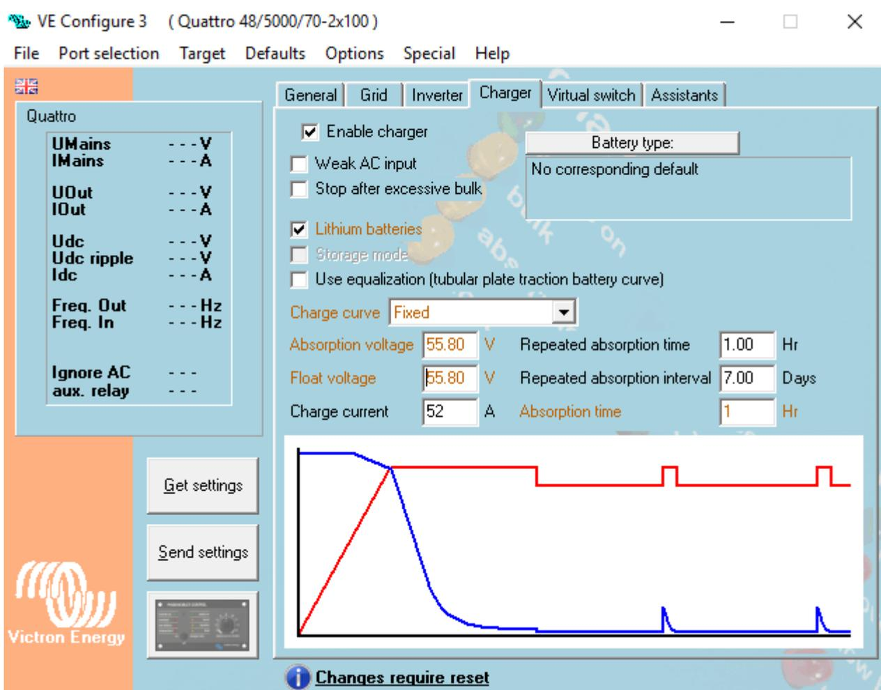
When setting up the ESS Assistant select LiFePO4 battery and enter the Ah value for the Lite (or the combination of Lite's for a parallel battery system) as per the Ah rating provided in the Lite specification sheet eg. Lite 5/4 = 100Ah.
