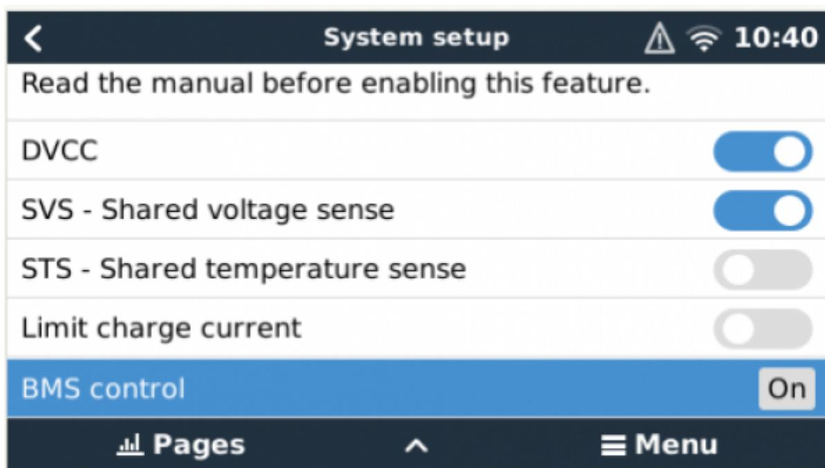
Freedom Lite (device list) → Parameters → Confirm that the Charge Current Limit and Discharge Current Limit are as per the Lite specifications (Note: if the battery is fully charged the CCL may be reduced. Check that the voltage target is within the range 54,1V to 55,8V (Note: below about 95% SoC the value reflected should be 55,7 or 55,8V. For a fully charged battery this value should range from 55,0V to 55,8V depending on the state of balancing of the cells in the Lite.
