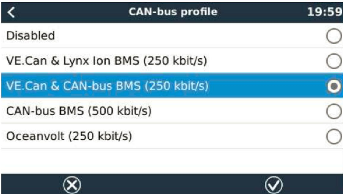
\* "VE CAN-bus & CAN-bus BMS (250 kbit/s)" should appear on the "CAN-bus(1) menu
