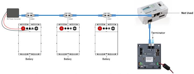
Note: Discover DC Power Converter and Lynx Gateway are Internally Terminated
