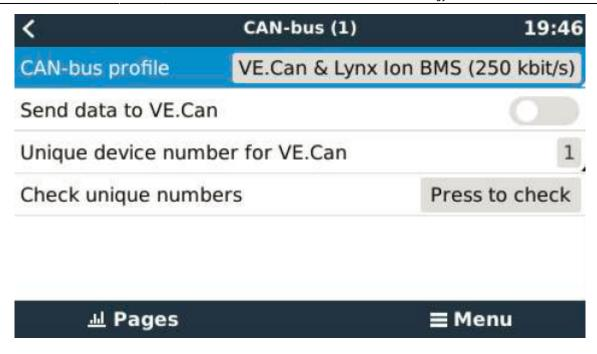
\* Within the "CAN-bus Profile" choose "VE CAN & CAN-bus"
