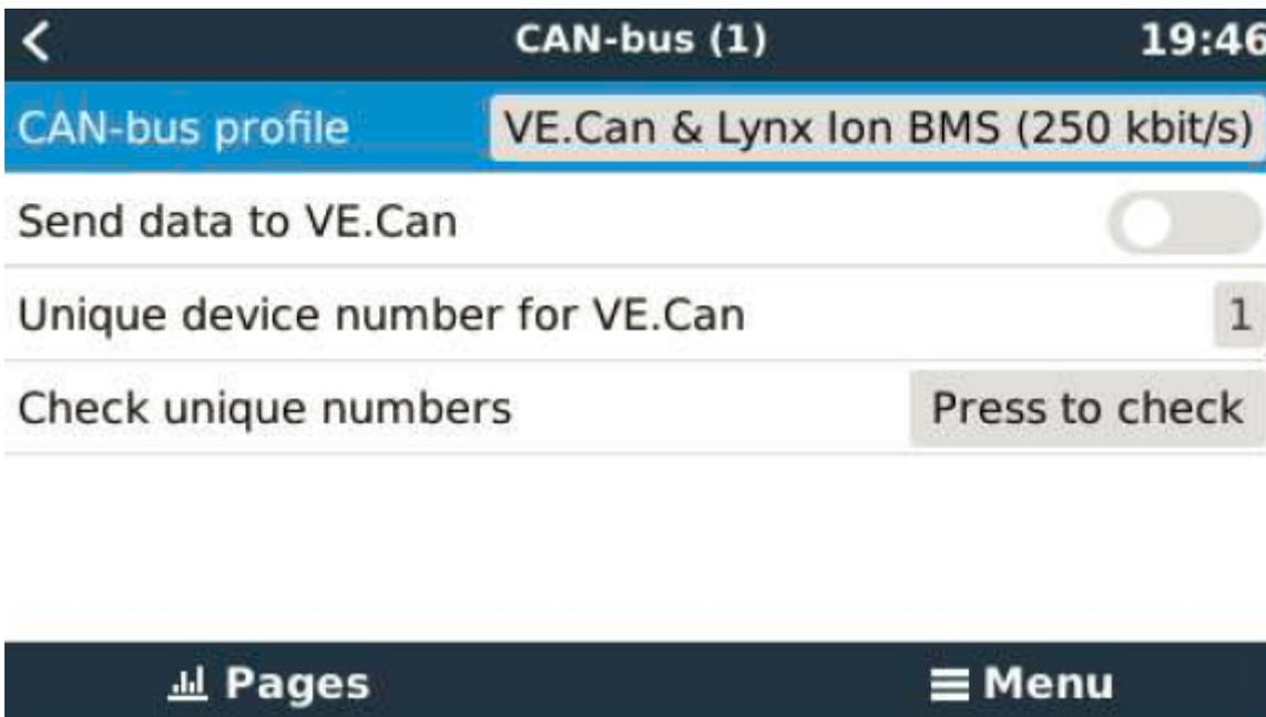
\* Within the "CAN-bus Profile" choose "VE CAN & CAN-bus"
