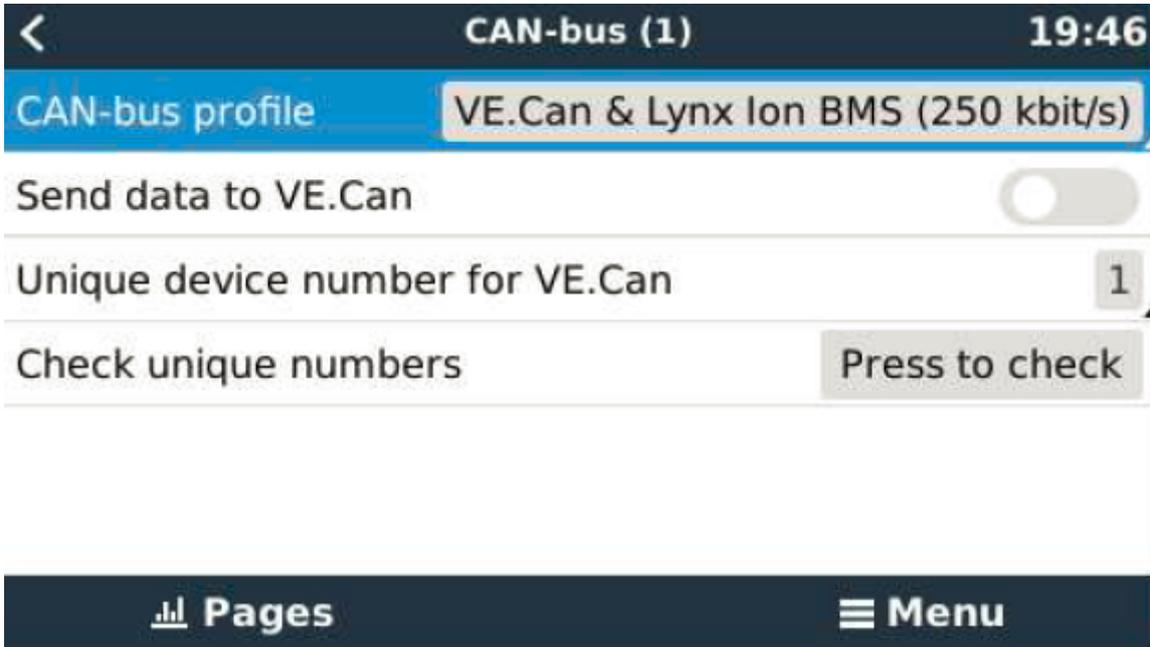
\* Within the “CAN-bus Profile” choose “VE CAN & CAN-bus”
