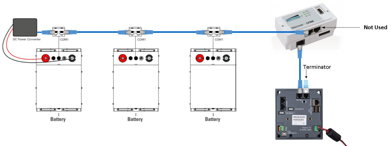
Note: Discover DC Power Converter and Lynx Gateway are Internally Terminated
