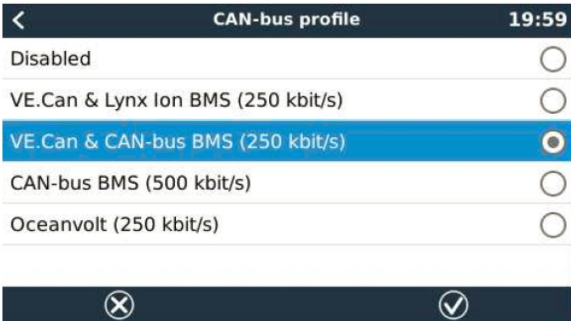
\* “VE CAN-bus & CAN-bus BMS (250 kbit/s)” should appear on the “CAN-bus(1) menu
