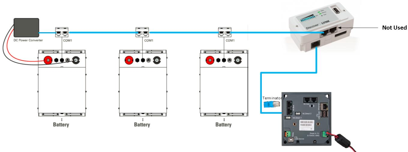
**NOTE:** Discover DC Power Converter and Lynk Gateway are internally terminated
