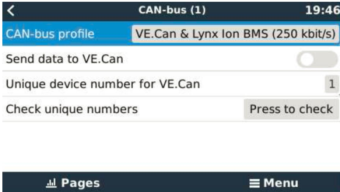
The screen shows the 'CAN-bus (1)' configuration. The top bar displays the title 'CAN-bus (1)', the time '19:46', and a back arrow. Below the title, 'CAN-bus profile' is set to 'VE.Can & Lynx Ion BMS (250 kbit/s)'. A toggle switch for 'Send data to VE.Can' is off. The 'Unique device number for VE.Can' is set to '1'. A button 'Check unique numbers' with the label 'Press to check' is present. The bottom navigation bar includes 'Pages' and 'Menu' buttons.
