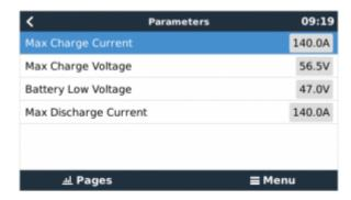
This parameters page is also a good place to check that all batteries are connected and working properly. In normal working conditions, for the 2.5 model, the charge current limit is  $\sim$ 35-50 A per cell. For example, 140A charge current limit ( 140 / 35 = 4 ) means there are 4 BYD battery cells connected.
