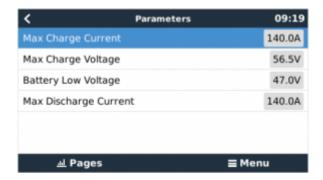
This parameters page is also a good place to check that all batteries are connected and working properly. In normal working conditions, for the 2.5 model, the charge current limit is  $\sim$ 35-50 A per cell. For example, 140A charge current limit ( 140 / 35 = 4 ) means there are 4 BYD battery cells connected.
