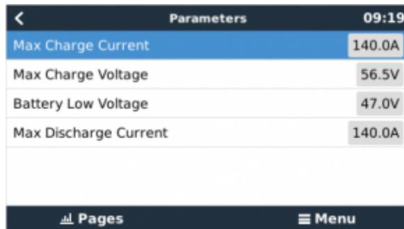
This parameters page is also a good place to check that all batteries are connected and working properly. In normal working conditions, for the 2.5 model, the charge current limit is ~35-50 A per cell. For example, 140A charge current limit (  $140 / 35 = 4$  ) means there are 4 BYD battery cells connected.
