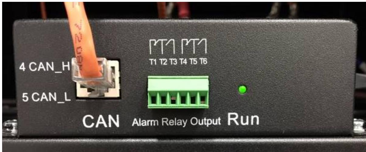
A blinking RUN led indicates an error. On the Victron system this is visible as a Max Charge Voltage of 42 V instead of 56.5 V.
