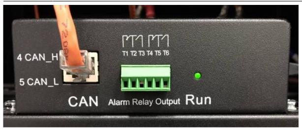
A blinking RUN led indicates an error. On the Victron system this is visible as a Max Charge Voltage of 42 V instead of 56.5 V.
