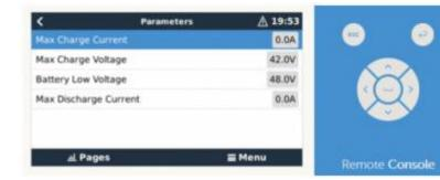
Also check that your are seeing the expected 35-40 A of discharge current per installed module.
