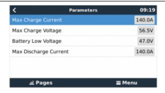
This parameters page is also a good place to check that all batteries are connected and working properly. In normal working conditions, for the 2.5 model, the charge current limit is 35A per cell. For example, 140A charge current limit (140/35 = 4) means there are 4 BYD battery cells connected. Note the discharge current limit figure has been increased in 2019 firmware versions - so it may appear slightly higher (eg 50A per cell).
