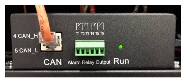
A blinking RUN led indicates an error. On the Victron system this is visible as a Max Charge Voltage of 42 V instead of 56.5 V.
