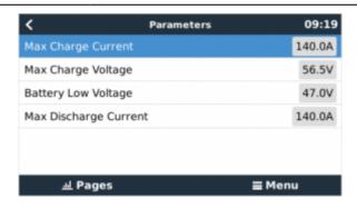
This parameters page is also a good place to check that all batteries are connected and working properly. In normal working conditions, for the 2.5 model, the current limit is 35A per cell. For example, 140A charge current limit (140/35 = 4) means there are 4 BYD battery cells connected. Note this figure has been increased in recent firmware versions - so it may appear slightly higher (eg 40A per cell).
