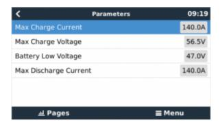
This parameters page is also a good place to check that all batteries are connected and working properly. In normal working conditions, for the 2.5 model, the current limit is 35A per cell. For example, 140A charge current limit ( 140 / 35 = 4 ) means there are 4 BYD battery cells connected.
