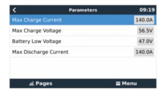
This parameters page is also a good place to check that all batteries are connected and working properly. In normal working conditions, the current limit is 35A per cell. For example, 140A charge current limit ( 140 / 35 = 4 ) means there are 4 BYD battery cells connected.
