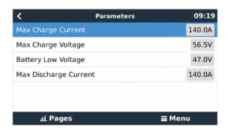
This parameters page is also a good place to check that all batteries are connected and working properly. In normal working conditions, the current limit is 35A per cell. For example, 140A charge current limit ( 140 / 35 = 4 ) means there are 4 BYD battery cells connected.
