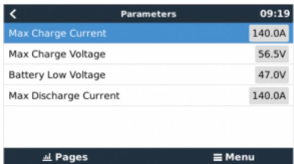
This parameters page is also a good place to check that all batteries are connected and working properly. In normal working conditions, for the 2.5 model, the current limit is 35A per cell. For example, 140A charge current limit (  $140 / 35 = 4$  ) means there are 4 BYD battery cells connected. Note this figure has been increased in recent firmware versions - so it may appear slightly higher (eg 40A per cell).
