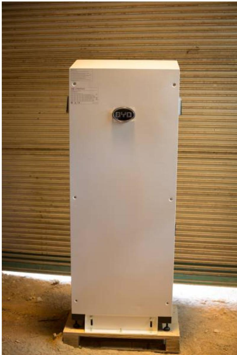
There is a foam seal all the way around the panel that should seal reasonably well when screwed on. The screws bound in their threads a little. Some remains of metal particles in the threads seemed to be the cause. The second unit we installed actually had one screw seize in the thread and needed
