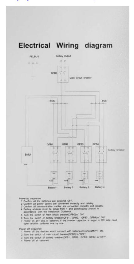
There are four individual breakers (one per battery unit) that are externally switchable and one main breaker (also externally switchable).
