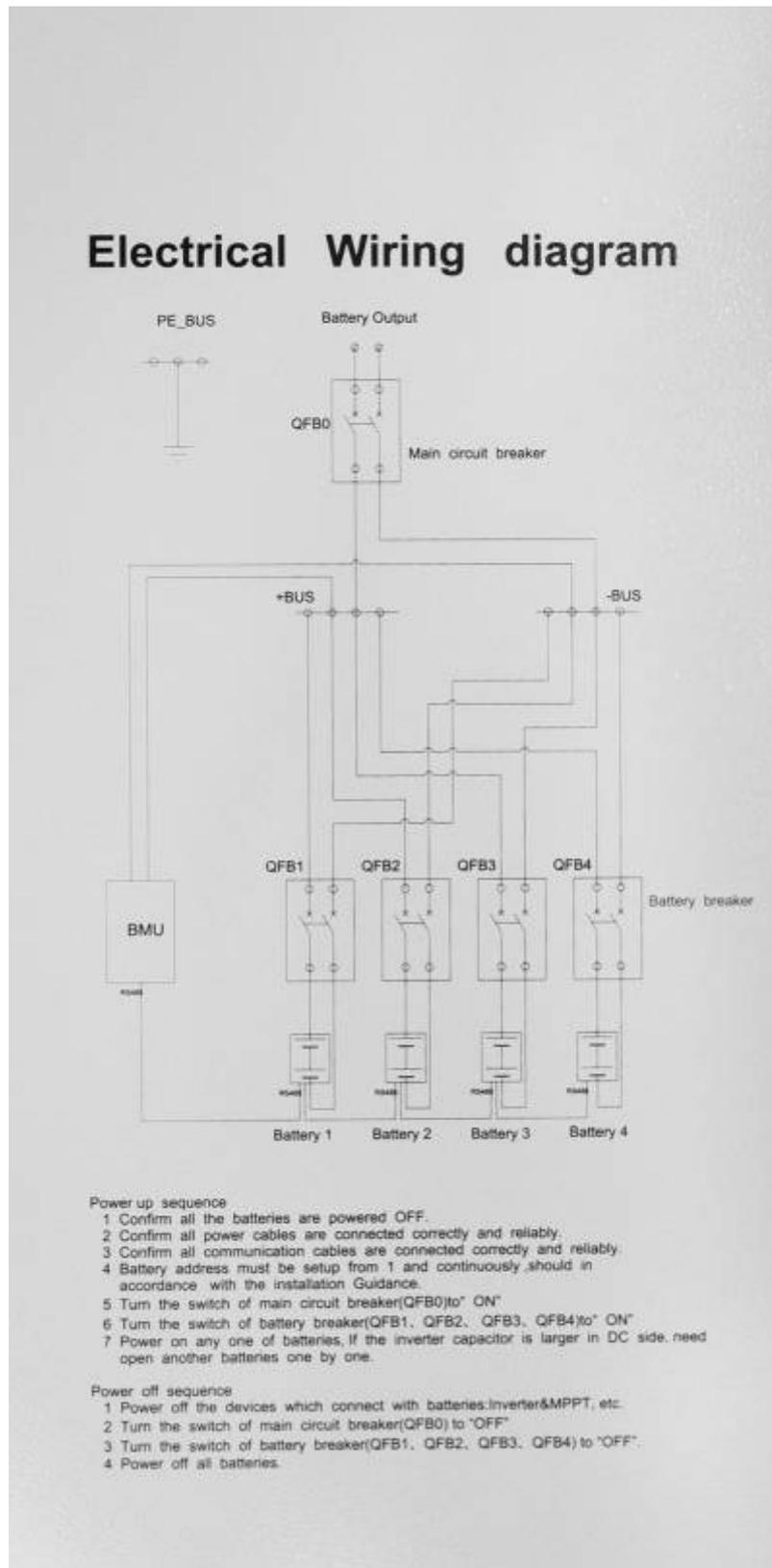
There are four individual breakers (one per battery unit) that are externally switchable and one main breaker (also externally switchable).
