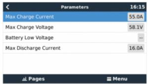
• Make sure to enable the *Synchronize VE.Bus SOC with battery* setting in the System Setup page in the CCGX: it will copy the State of Charge as reported by the BMZ ESS to the Multi or Quattro, making Hub-4 work with that SOC.
