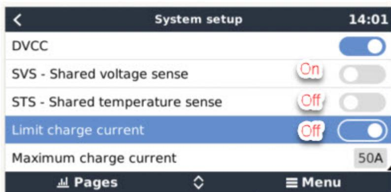
Shared Voltage Sense (SVS) Works with VE.Bus devices and VE.Direct Solar Chargers.
