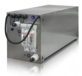
No RJ45 cable is supplied for this connection . Plug the CCGX/VenusGX side of the cable into one of the VE.Can sockets on the back of the CCGX/VenusGX. Plug the other end into the battery at one of the RJ45 CANbus ports. A VE.Can terminator is not nescessary for the other VE.Can socket on the CCGX/VenusGX. Without properly connecting this cable, the battery will stop charging/discharging after several minutes. Also, the battery will not show up on the display of the CCGX/VenusGX. ==== 4.1 Charge
