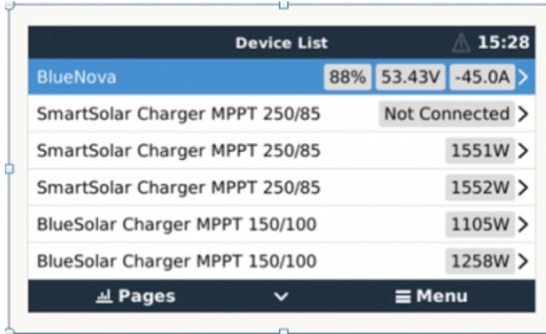
If you have multiple batteries, a single entry will show up, which represents all batteries. The parameters option within the battery page shows the actual battery charge and discharge limits. ===== 6. Configure MPPT ===== - Disable Autodetect voltage - Set Battery voltage to 48V. It is recommended to make these settings using the VictronConnect App and Bluetooth. - All latest GX devices applicable.
