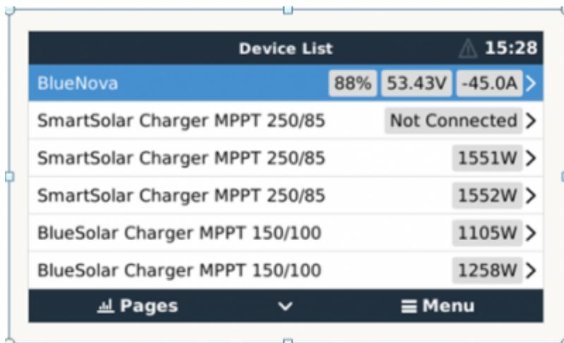
If you have multiple batteries, a single entry will show up, which represents all batteries. The parameters option within the battery page shows the actual battery charge and discharge limits.
