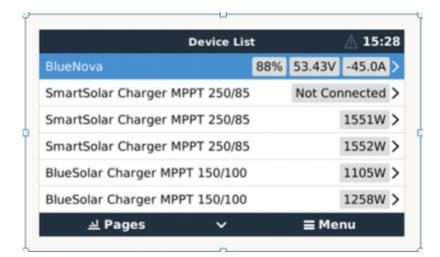
If you have multiple batteries, a single entry will show up, which represents all batteries. The parameters option within the battery page shows the actual battery charge and discharge limits.
