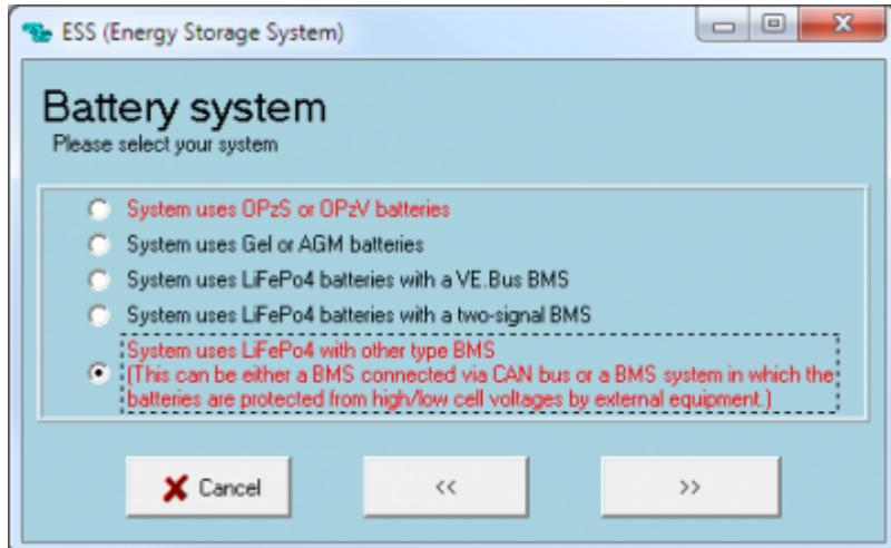
5. Color Control GX Configuration Enable the CAN-bus BMS Service in the CCGX. Menu path: Settings → Services → CAN-bus BMS. Note that this changes the function of a VE.Can port: it is not possible to connect both VE.Can products and a Bluenova battery together.
