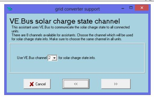
In a 3 Phase system, each Phase Master unit must have the Grid Converter Support Assistant added.
