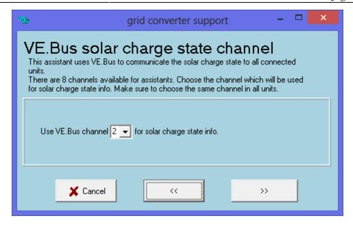
For Solar Charging Current, each Phase Inverter/charger must use its own Channel, see below the screen showing this setting.
