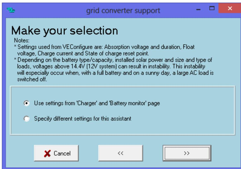
This setting is to reset the Grid Inverter once it has been switched off, reset into sleep mode. This happens when there is no load connected to the system and the battery bank is fully charged.
