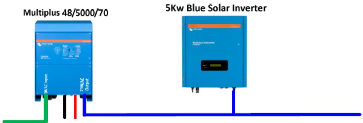
It is very important to ensure the loads are well balanced in a 3 phase system with Grid Inverters. Careful attention must be paid to all Cabling DC and AC Cabling; the wire size must be rated correctly. The AC cabling must also be of the same length throughout from the Input into the Inverter/chargers and from the Output to the Grid Inverter/s and to the Distribution Board.
