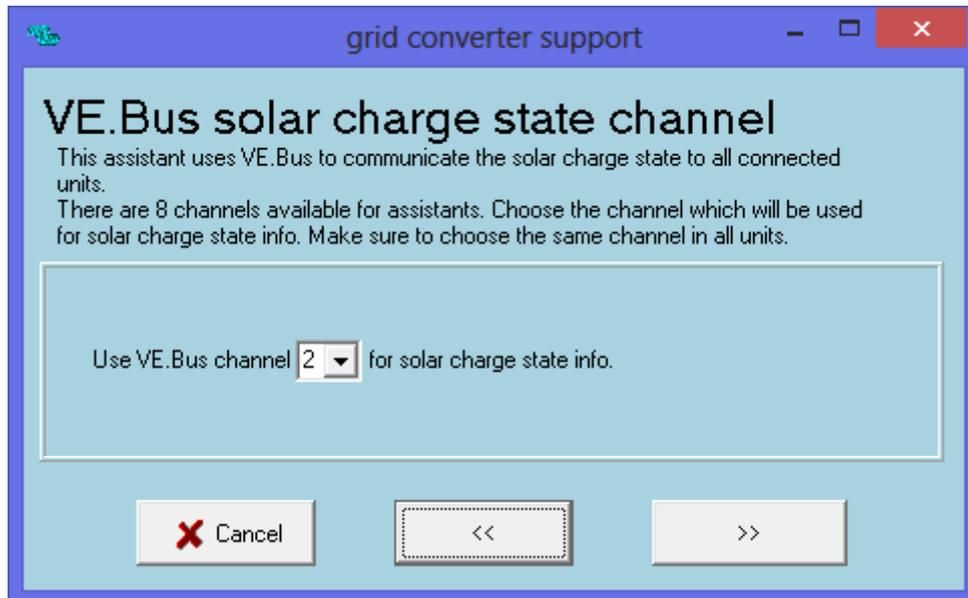
For Solar Charging Current, each Phase Inverter/charger must use its own Channel, see below the screen showing this setting.
