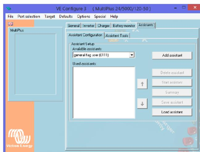
Before the setup using the Assistant can be done it is important to know at what frequency will the Grid Inverter go into sleep mode, the shutdown Hz level shut not be used to prevent any unnecessary on/off switching. The sleep mode keeps it on and when set into sleep it will provide power very quickly thereafter.
