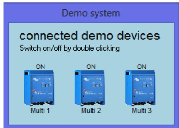
When making your VE Configure 3 settings in the master ensure all settings except the Assistant settings are sent to all units. Thereafter you make your assistant settings in the master and send it only to the Master. The image below is the only screen that is added from a single unit installation for the assistant. The default channel value is the correct setting.
