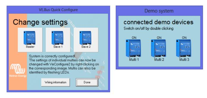
When making your VE Configure 3 settings in the master ensure all settings except the Assistant settings are sent to all units. Thereafter you make your assistant settings in the master and send it only to the Master. The image below is the only screen that is added from a single unit installation for the assistant. The default channel value is the correct setting.
