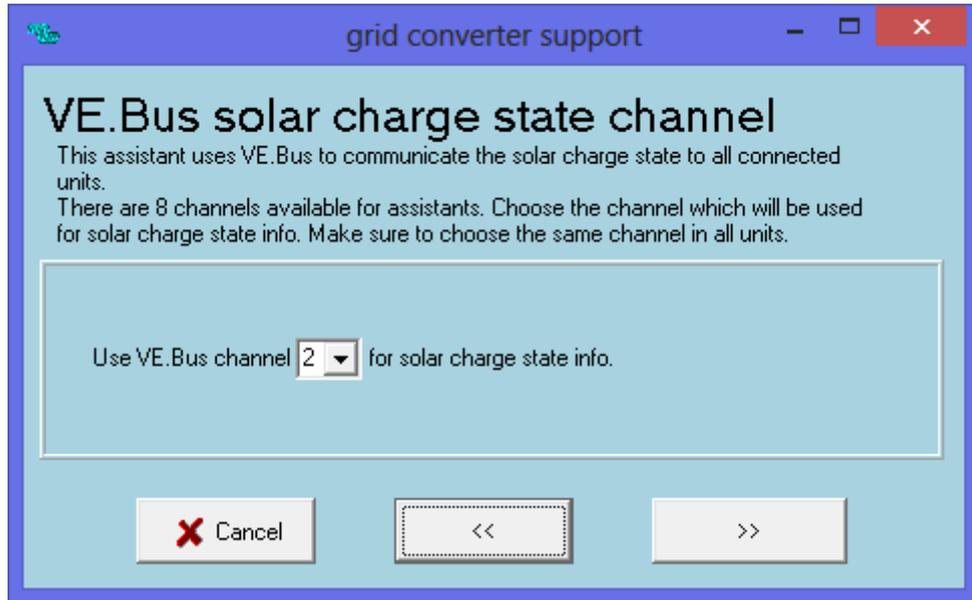
In a 3 Phase system, each Phase Master unit must have the Grid Converter Support Assistant added.
