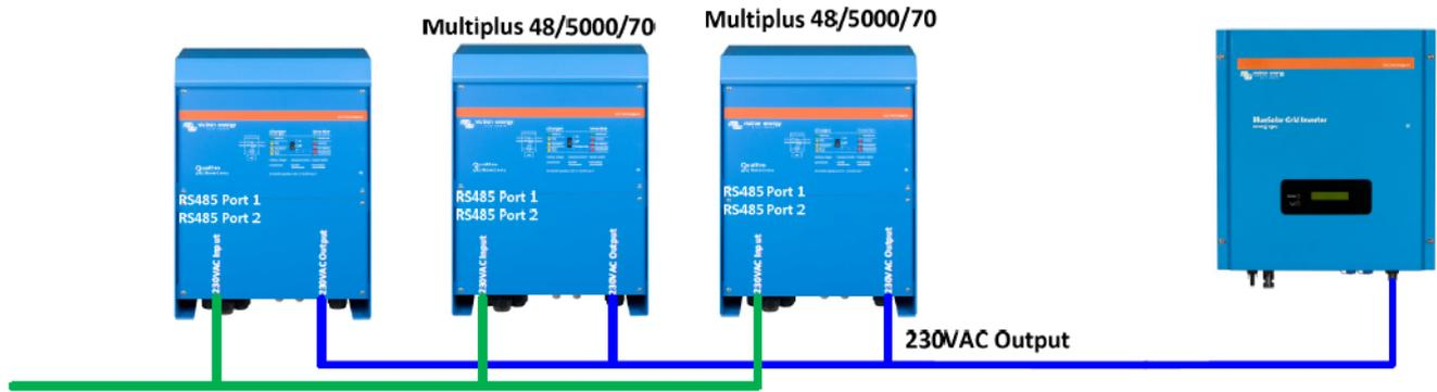
Careful attention must be paid to all Cabling DC and AC Cabling; the wire size must be rated correctly. The AC cabling must also be of the same length throughout from the Input into the Inverter/chargers and from the Output to the Grid Inverter/s and to the Distribution Board.
