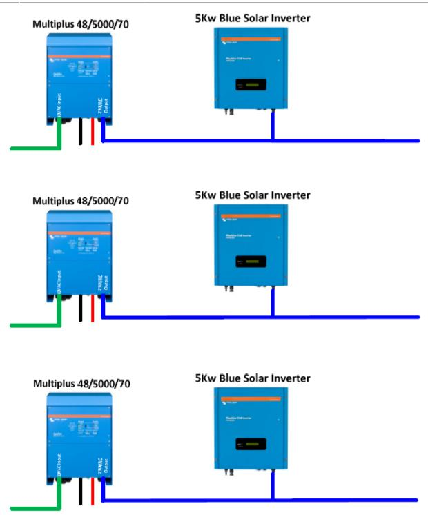
It is very important to ensure the loads are well balanced in a 3 phase system with Grid Inverters. Careful attention must be paid to all Cabling DC and AC Cabling; the wire size must be rated correctly. The AC cabling must also be of the same length throughout from the Input into the Inverter/chargers and from the Output to the Grid Inverter/s and to the Distribution Board.
