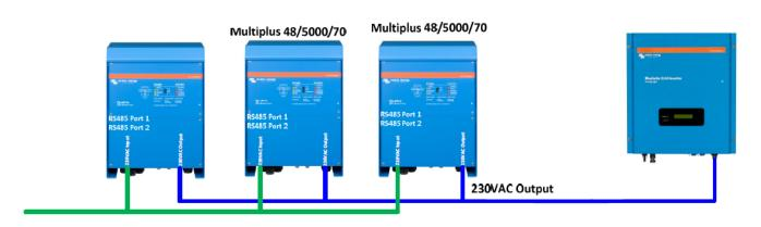
Careful attention must be paid to all Cabling DC and AC Cabling; the wire size must be rated correctly. The AC cabling must also be of the same length throughout from the Input into the Inverter/chargers and from the Output to the Grid Inverter/s and to the Distribution Board.
