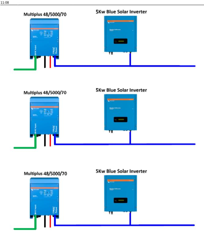
It is very important to ensure the loads are well balanced in a 3 phase system with Grid Inverters. Careful attention must be paid to all Cabling DC and AC Cabling; the wire size must be rated correctly. The AC cabling must also be of the same length throughout from the Input into the Inverter/chargers and from the Output to the Grid Inverter/s and to the Distribution Board.
