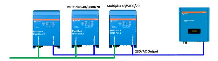
Careful attention must be paid to all Cabling DC and AC Cabling; the wire size must be rated correctly. The AC cabling must also be of the same length throughout from the Input into the Inverter/chargers and from the Output to the Grid Inverter/s and to the Distribution Board.
