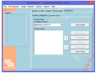
Before the setup using the Assistant can be done it is important to know at what frequency will the Grid Inverter go into sleep mode, the shutdown Hz level shut not be used to prevent any unnecessary on/off switching. The sleep mode keeps it on and when set into sleep it will provide power very quickly thereafter.
