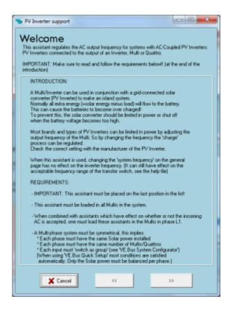
Use this Assistant in systems with a grid-tie PV inverter connected to the AC out of a Multi or Quattro, where ESS is not applicable. Off-grid systems, and in certain cases also backup systems.
