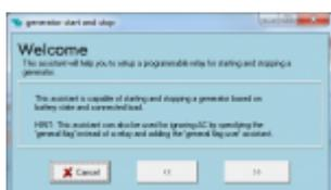
Automatically start and stop a generator based on battery state of charge and actual load of a system. Note that automatic genset start/stop functionality is also available on the Virtual switch tab in VEConfigure, which is easier to work with.
