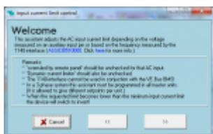
Automatically set the input current limit to a predefined value based on the state of an aux input or rpm measured with the 1140 interface. Used in the following systems:
